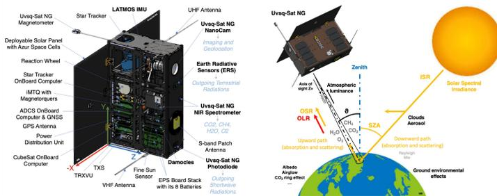
Figure 9. Computer-aided design of the Uvsq-Sat NG CubeSat.
