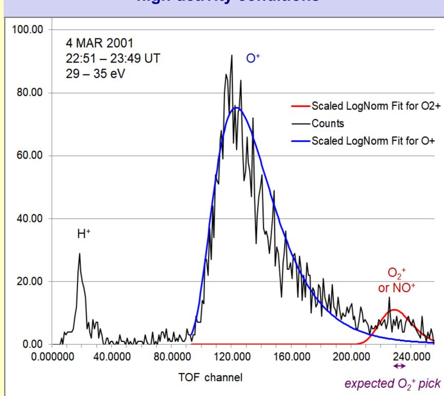
Time-of-flight spectrum for the low-energy ions detected by CIS onboard Cluster-C1 during the 4 March 2001 event, where two interplanetary shocks struck the magnetosphere, followed by a strongly southward oriented IMF . The spacecraft was over the southern polar cap at  $R = 7 R_E$ . Observation of an upwelling ion population containing H<sup>+</sup>, O<sup>+</sup> and O<sub>2</sub><sup>+</sup> or NO<sup>+</sup> ions.
