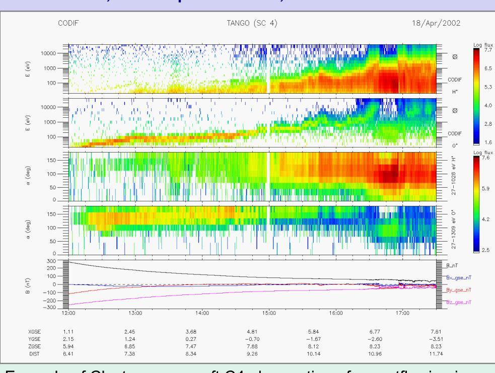
Example of Cluster spacecraft C4 observation of an outflowing ion beam, detected by the CIS-CODIF instrument above the northern polar cap during an outbound orbit. The outflowing ions population corresponds to the dominant >90° pitch angle population.
