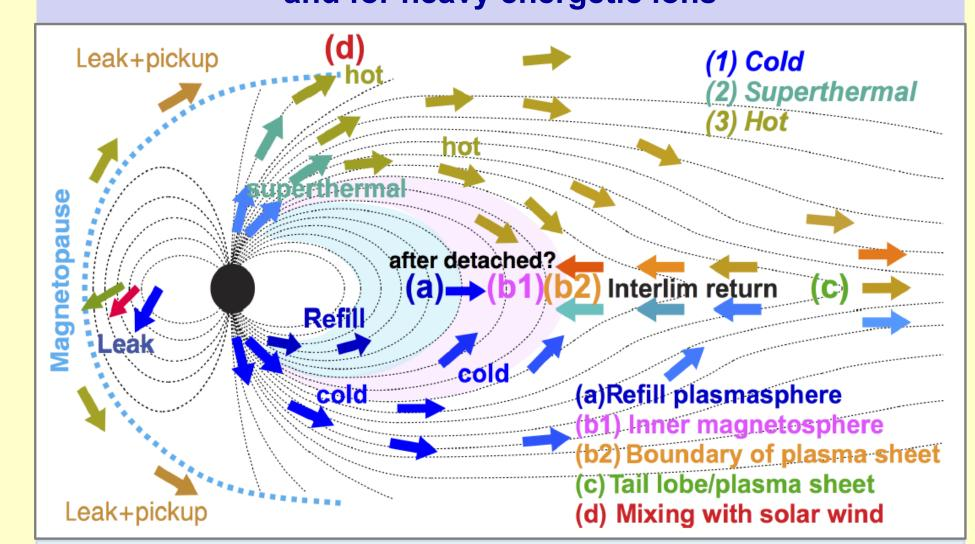
Schematic representation of the circulation of outflowing ions in the magnetosphere and their destination.
